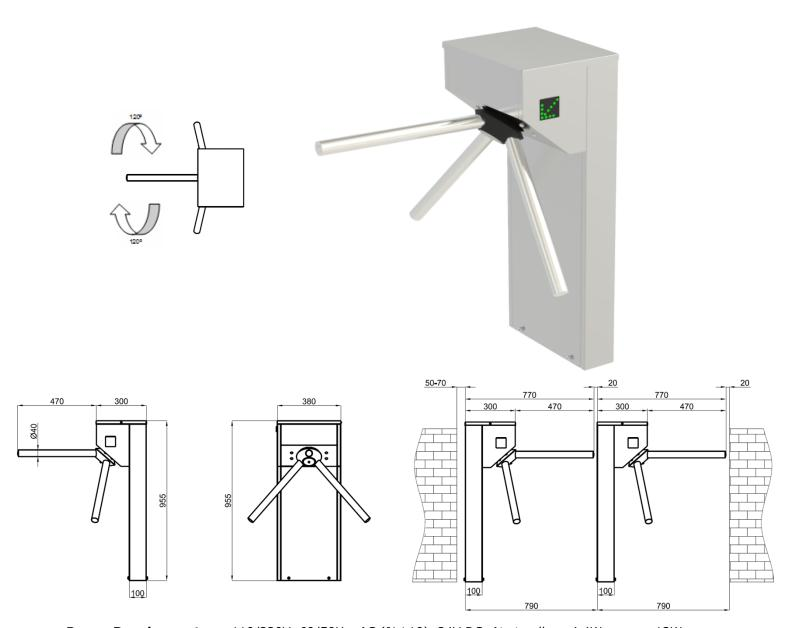
**Power Requirements**: 110/220V. 60/50Hz. AC (% $\pm 10$ ), 24V DC. At standby  $\sim 4,4$ W. max.  $\sim 12$ W.
